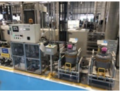
Recovering refrigerant in the production process
