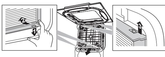
**3** Clean the air filter. Use a vacuum cleaner or wash with water. If the air filter is very dirty, use a soft brush and neutral detergent.
