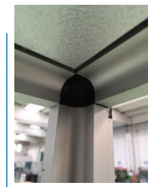
Fig 1: Internally Rounded Profile
